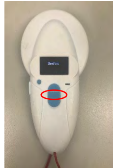
Figure 28: PIT tag application sites (red circles), and PIT tag scanner with « reading » button highlighted - rectangular middle button.
